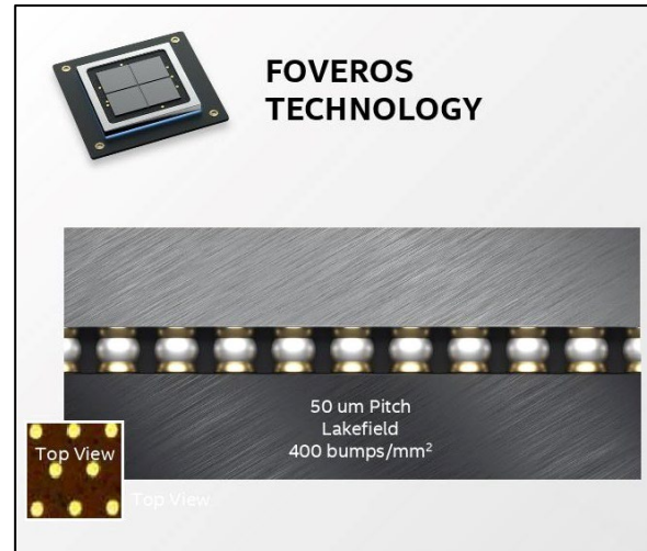
Micro-Bumping, Intel 50um pitch demonstrated
